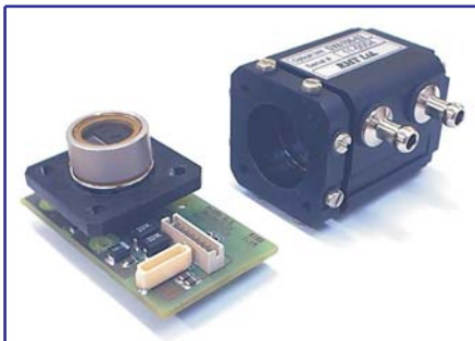
Fig. 3.2. DX6106 Optical Unit with optopair detached
