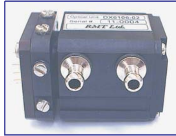
Fig. 3.4. DX6106.C40 gas sampling cell
